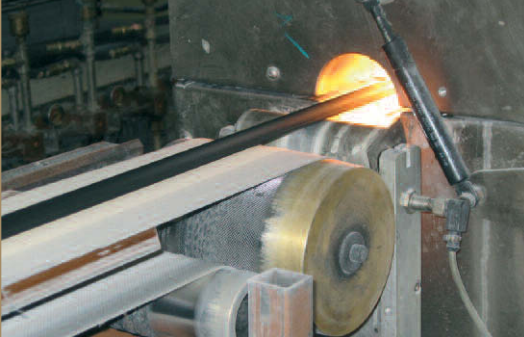
Rubber profile curing
