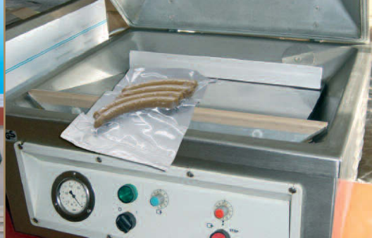
Vacuum packaging - heat shrinking
